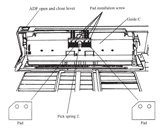
Figure 5.8 Removing the pad
